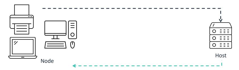
A node refers to any device on the network. (Examples: computer, routers, printers)  A host is a node that has a unique function. Other devices connect to nodes so they can access data or other services. (Example: server)
