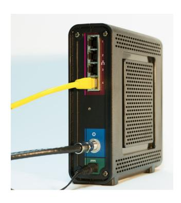
An example of a modem, where the coaxial cable connects from internet service provider (ISP) to your modem. Depending on the modem, you will then have wireless internet or connect it to a router.
